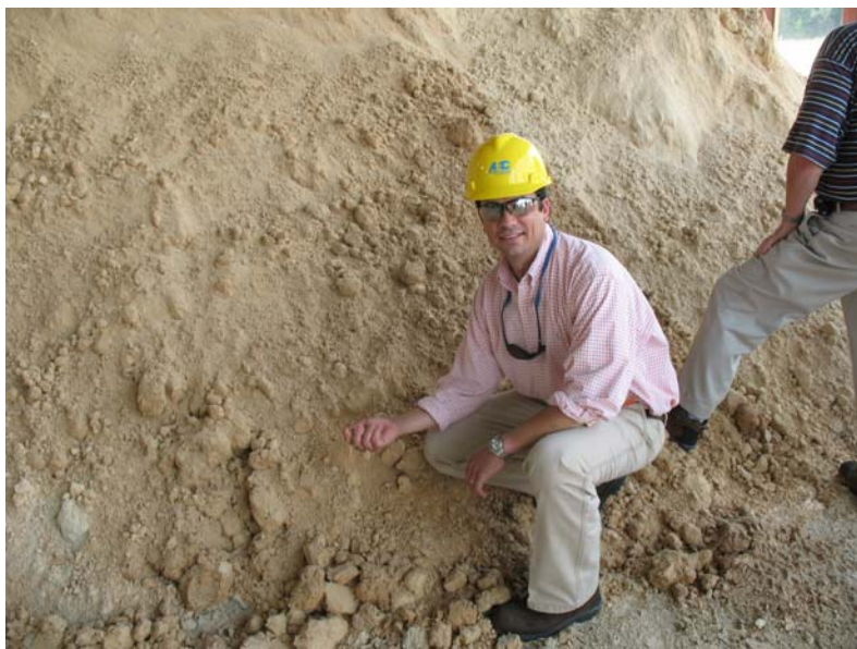
A stockpile of FGD gypsum produced by Power South Electric Cooperative's Charles R. Lowman Power Plant near Leroy, Alabama.
